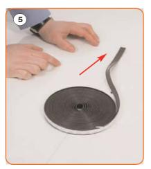
Attach magtape to both vertical sides of each clear acetate panel.
