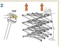
Assemble frame with the yellow coloured hookstuds at the top.
