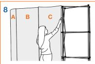
Working to the right take panel 'B' and hook it on to the yellow nodes at the top so it butts up against panel A on the left and takes up the other half of the magnetic bar. Work across to the right adding panels until you get to the opposite D-end panel which will wrap around to the rear as before.
