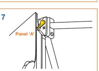
Start with D-end panel 'A' on the left end of the frame and hook it on the yellow node at the front top of the frame aligning it to outer half of the magnetic bar. Bring the panel around to the rear of the frame and hook it on to the yellow node at the back so it creates a rounded end and hides the side framework.
