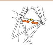
Push the locking bars together until they attach magnetically.
