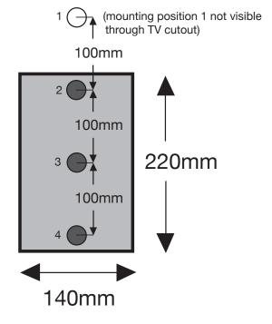
There are four mounting positions on the pole. The first hole cannot be used but the other three can. Position three is the default setting but if needed positions two and four can be used.
